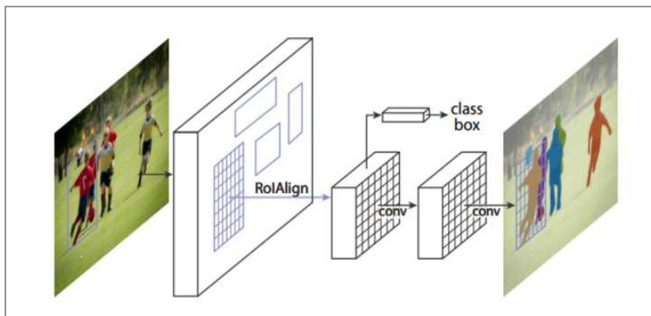
Figure (2): Mask RCNN architecture, Source: Esri
